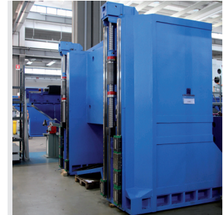
Cast iron structure
