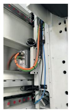
Transversal axis frame (Y axis) composed of a duly optimized crossbeam with wide-section guides and preloaded rollers for saddle movement
