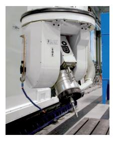
Jobs LINX CUBE is the ultimate high-performance 5-axis milling machine from LINX linear motors gantry family: a new model at the top of performance able to reduce machining time increasing machining quality.
