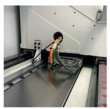
A conditioning system by cooling liquid provides thermal stability for both the primary motors and the structures underneath the secondary motors, guaranteeing a very high accuracy
