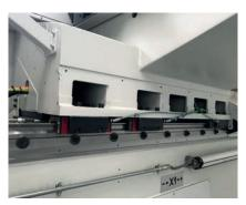
Large-size X-axis bedplates featuring 2 widesection guides and preloaded rollers on each side
